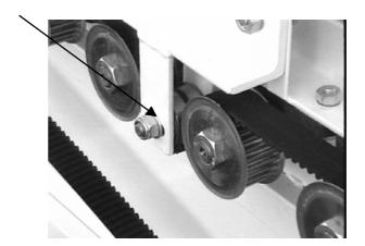
To replace rollers, loosen the tension roller and remove the toothed belt drive. Remove the lock-nut and toothed drive gear. The bearings and rollers can now be removed. The rubber discs and nylon rings can be replaced after fitting a stop ring on the rubber roller.
